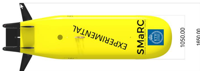
AUV LoLo (dimensions in mm)
