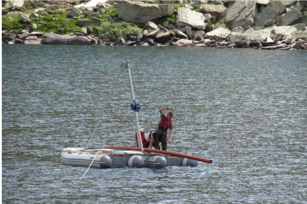
Fig. 3. The assembled raft and Nesje coring system that was used in the European Alps.
